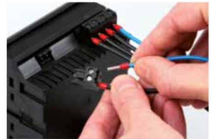
Fig.: Pluggable screw terminals for easy connection
